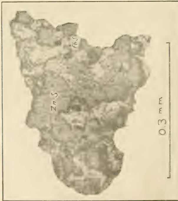
A. A 65-MESH PARTICLE OF ORE 3, SHOWING ASSOCIATION OF THE GALENA AND ZINC BLENDE.
